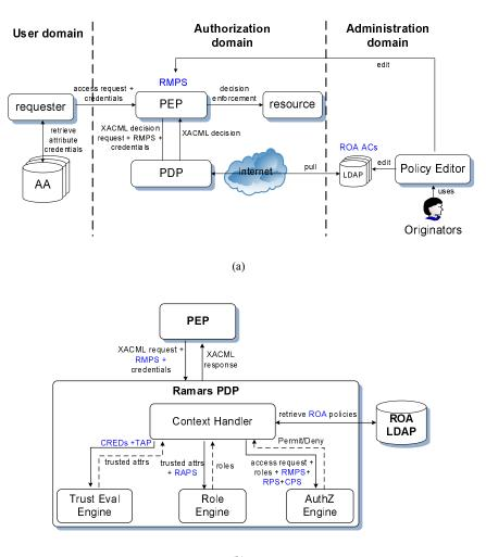
Figure 1 RAMARS system architecture (a) RAMARS architecture (b) RAMARS PDP and policy evaluation (see online version for colours)
