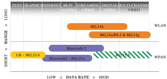
Figure 5: Current and proposed WLAN & WPAN standards.
