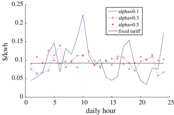
**Fig. 5** SRP RTP fluctuation (detached type only)
