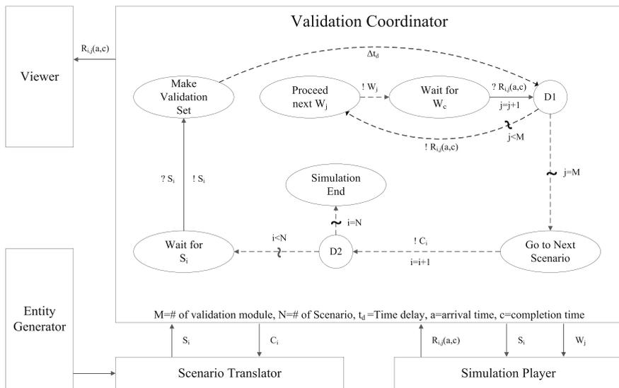
Fig. 2 Validation coordinator using DEVS formalism
