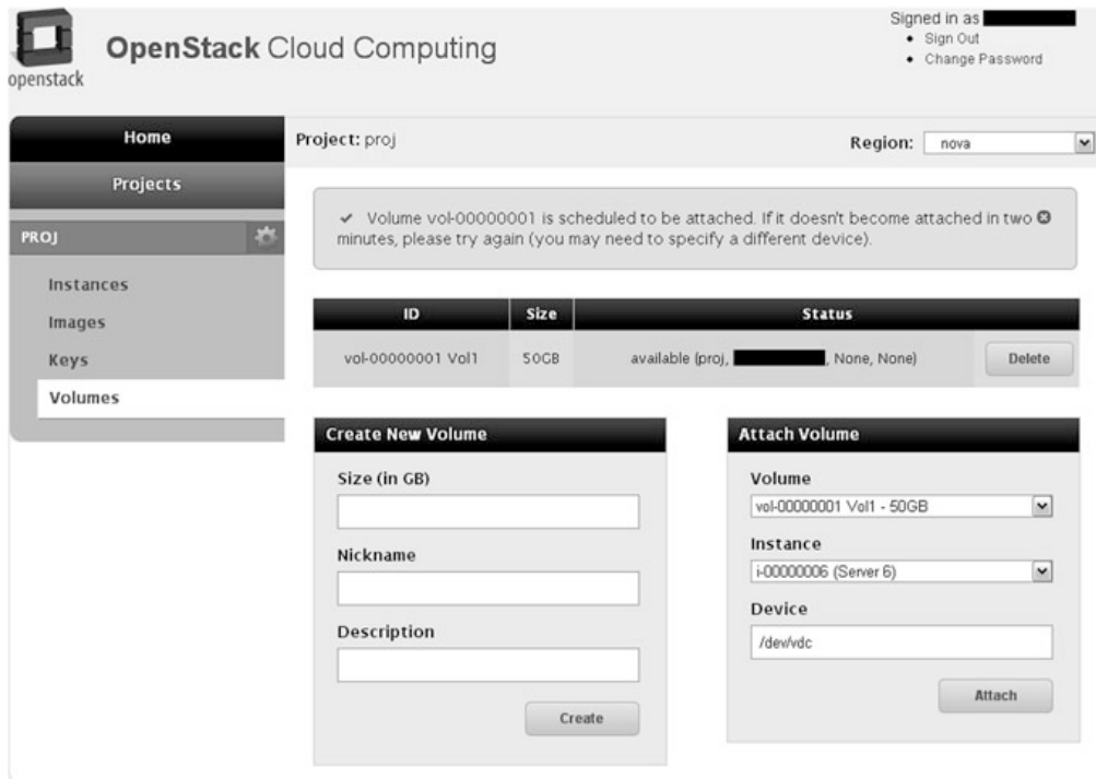
Fig. 12.10 A screen shot of the OpenStack dashboard immediately after connecting a volume to a running instance as /dev/vdc
